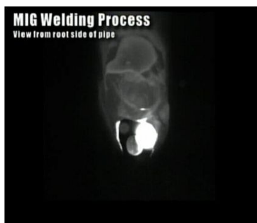
Fig. 2.15 Short Circuit Transfer
